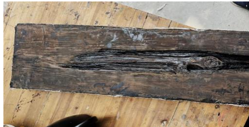
Figure 7. Elm wood (with its own incomplete texture), framed with linen cloth, and painted with raw lacquer.
