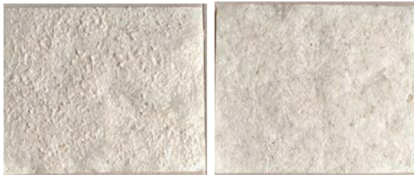
Figure 2: Sugar palm fruit shell paper: front side (left) and back side (right).
